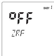
2 **Parent unit:** Press the **"M"** button two times. The display changes from **SLEEP TIMER** to **ZRF**.
